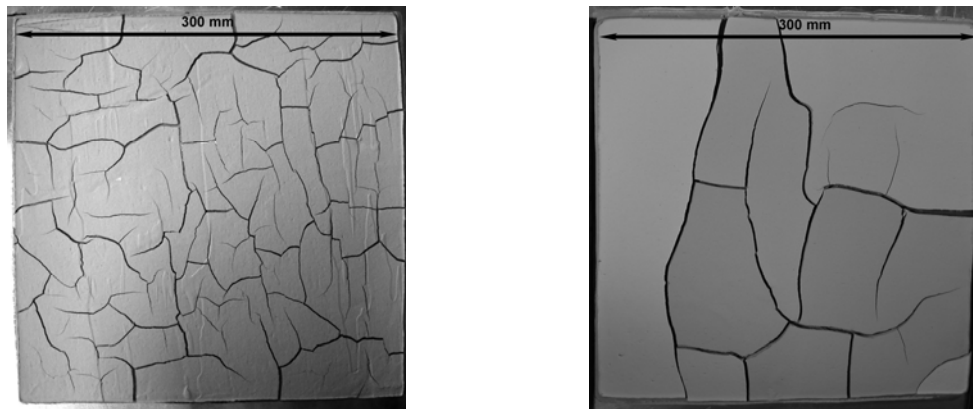
Figure 2- 2D desiccation tests, final stage of cracking (left, samples 4 mm in height, right, samples 12 mm in height)
